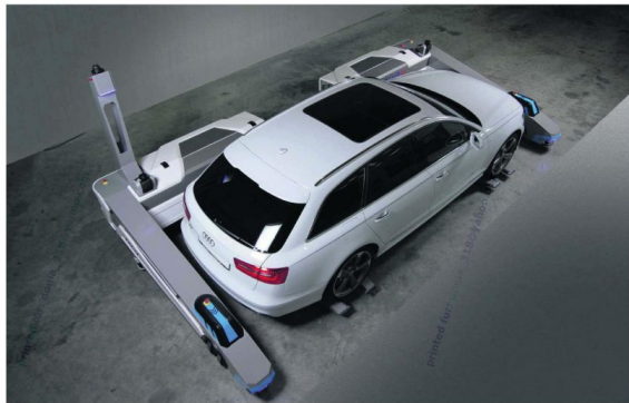
GreenParking's Robot Ray is tailored to fit into existing structures so car parks do not need alterations. Courtesy GreenParking
